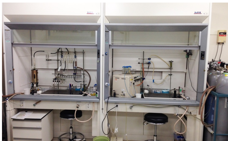
An apparatus for the gassing anoxic gases (in the left hood) and a gas exchanger (gassing manifold) equipped with a vacuum pump (in the right hood)
